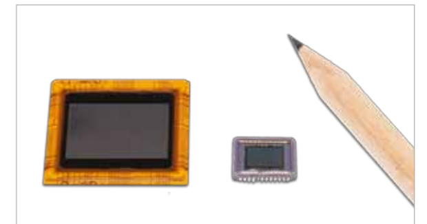
The PEN image sensor in comparison with the average sensor for compact cameras.
